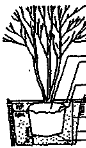
TYPICAL ORNAMENTAL TREE PIT DETAIL SCALE 1/4" = 1'-0"
