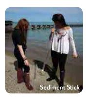
Show students the sediment stick, which is one tool used to measure turbidity.
