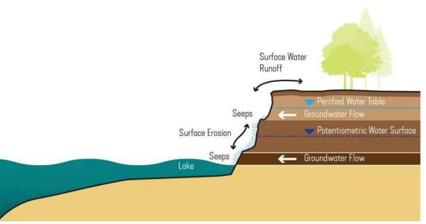
Figure 2.5 Stormwater & Groundwater Bluff Instability
