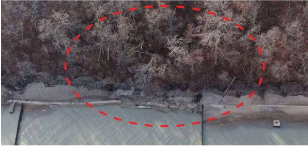
Figure 2.27 Aerial Photo of Bluff Failure, Late Fall 2020.
