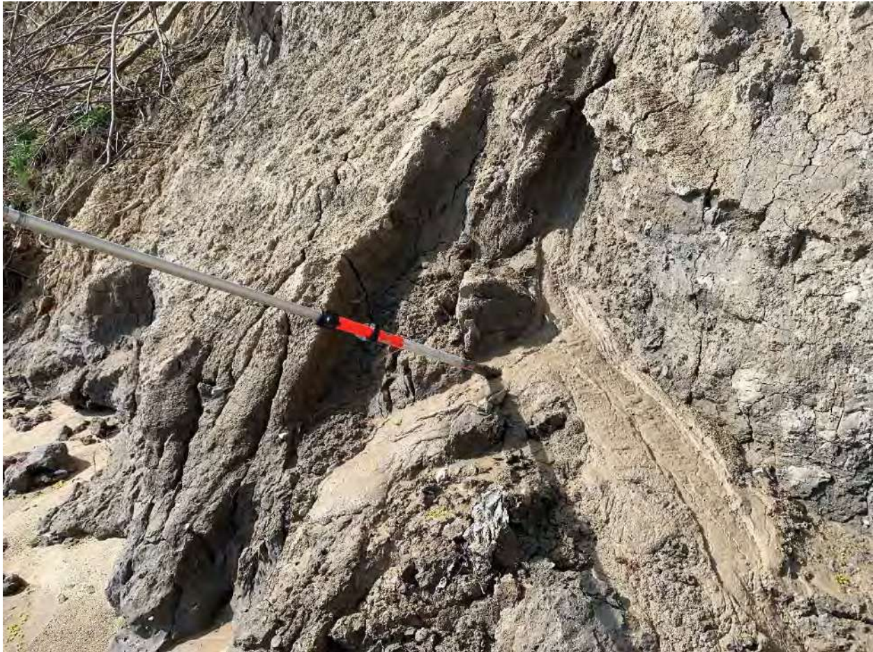
Figure 2.31 Liquifying soil seeping out the face of the bluff along the beach due to excessive soil saturation.
