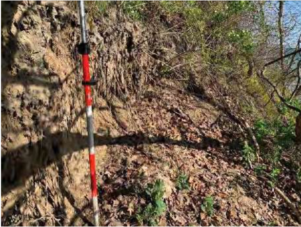
Picture 1: Vertical drop due to slope failure.
