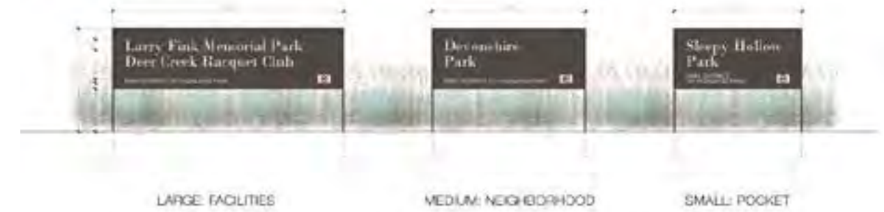
OPTION 2: PAINTED METAL SIGN + WEATHERED STEEL FRAME
