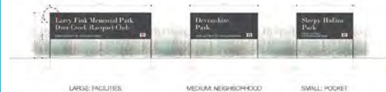
OPTION 3: PAINTED METAL SIGN WITH PAINTED STEEL FRAME CHARCOAL-GREY OR BLUE-GREY
